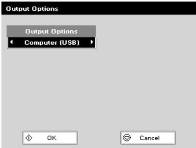
Select how the data are send. Options are **Computer (USB)** or **None**. Press **OK** to store the settings and return to the **Utilities** folder **OR** press **Cancel** to return to the **Utilities** folder without storing the settings.
