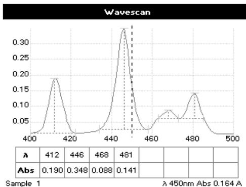
**Peak Detect on Zoom:** Determines whether peaks are re-assessed and tabulated when the user zooms into a region of the wavescan. If **Off**, leaves the peak detection as determined on the un-zoomed display.
