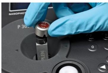
**Step 4** Make sure that for the measurements the lid fits exactly onto the positioning supports mounted to the body of the cell. Take measurement. **Remember** to consider the lid factor in your instrument software. Please refer to the NanoPhotometer® P-Class User Manual for detailed information.
