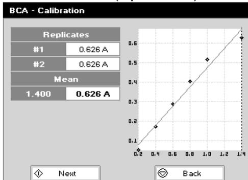
**Calibration Screen (replicates on)**
