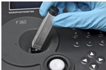
**Step 1** Insert the NanoPhotometer® P-Class Submicroliter Cell into the cell holder with the cell windows facing the light beam. We recommend facing the Implen logo to the front. The light beam is directed from RIGHT to LEFT as indicated with small arrows. Insert the NanoPhotometer® P-Class Submicroliter Cell always in the same direction.
