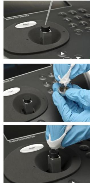
Please note that all kind of high concentrated acids and bases are not recommended. It is recommended to wipe off every sample immediately upon completion of a measurement. For more specific solvents, please contact the Implen support team ([support@implen.de](mailto:support@implen.de)) to check the compatibility.
