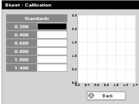
**Step 13** **Calibration Screen (replicates off)** This shows the calibration values and allows standards to be measured. Insert the reference sample. Press **Blank** key. This will be used for all subsequent samples until changed.
