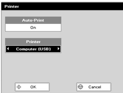
**Step 1** Select whether **Auto-print** is on or off using the left and right arrows. When auto-print is “on” the results are automatically printed after a measurement is taken. When it is set to “off”, printing has to be initiated manually. This can also be set using the **Options** key in each application or method. The default is OFF.
