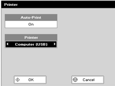
**Step 1** Select whether **Auto-print** is on or off using the left and right arrows. When auto-print is set as “on” the results are automatically printed after a measurement is taken. When setting is “off” printing has to be initiated manually. This can also be set using the **Options** key in each application or method. The default is OFF.
