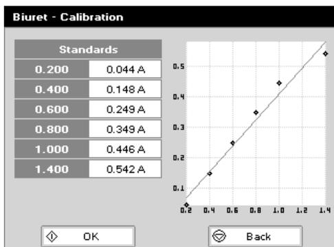
**Step 15** Repeat for all standards. A graph will display the results and the fitted curve as the measurements are made. Use the up and down arrows to select a standard to be repeated if a poor reading has been obtained. Use C to clear the previous reading.
