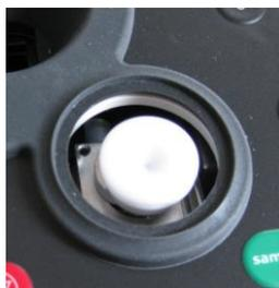
2. Place the new gaiter in the gap and in a first step place inner flute and in the second step the outer flute.
