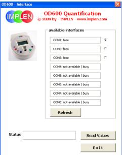
**Step 4:** Click the "Read Values" button. The message "Press 'OK' and then press 'print' on device within 20 seconds" will appear. Press OK and then press the recall/print button on your OD600 DiluPhotometer<sup>TM</sup>.
