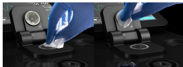
**Note:** Make sure that the metal contact face (around the measurement window and the mirror) is clean.
