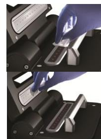
11. Apply samples to the illuminated sample windows on pedestal and press the sample button to initiate the measurement.
