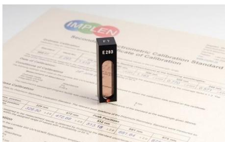
The certified didymium glass filter can be used to verify the wavelength and photometric accuracy of the NanoPhotometer® cuvette applications.
