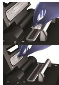
12. Apply samples to the illuminated sample windows on pedestal and press the sample button to initiate the measurement.
