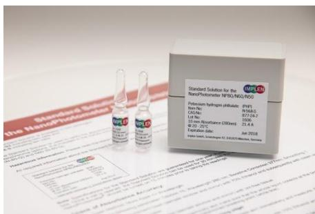
The NanoPhotometer® is recalibration free therefore it is not necessary to review the photometric accuracy on a regular basis. If the SOPs of a laboratory require a routine control of the photometric accuracy standard solutions can be used.
