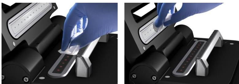
**Note:** Make sure that the metal contact face (around the measurement window and the mirror) is clean.
