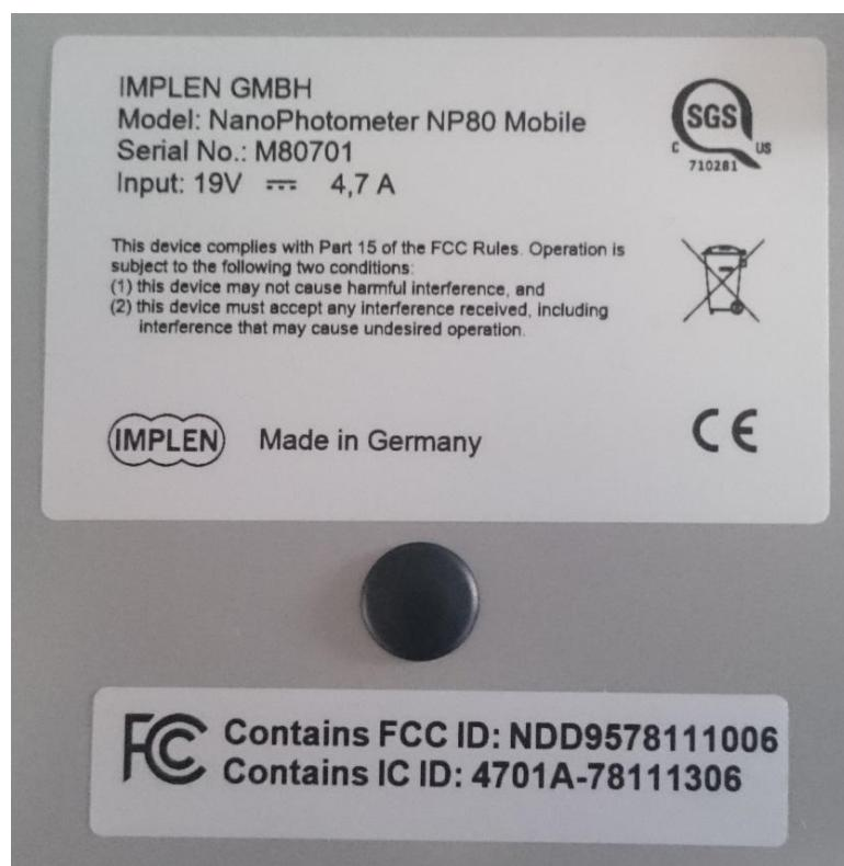
Model name, device serial number and FCC ID are located on the identification plate on the bottom of the instrument.
