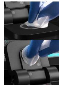
10. Apply sample to the sample window on pedestal and press the sample button to initiate the measurement.
