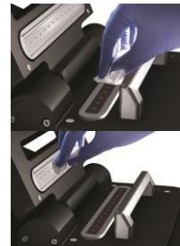
13. Apply samples to the illuminated sample windows on pedestal and press the sample button to initiate the measurement.
