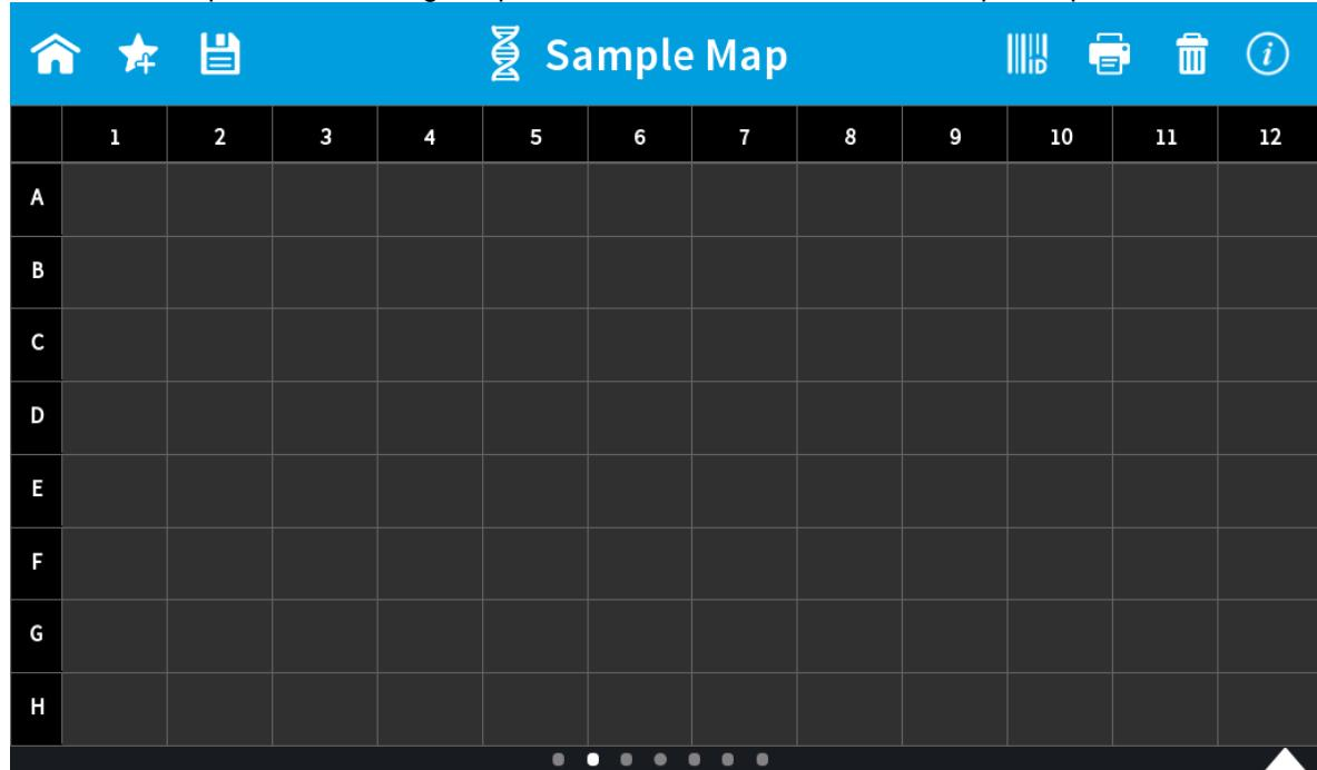
The sample map offers the possibility to select cells and define sample IDs for measurements. It is not necessary to make any selection. If cells are left empty without defined sample IDs for horizontal or vertical sample loading, all 12 positions for horizontal loading or all 8 positions for vertical loading are measured.
