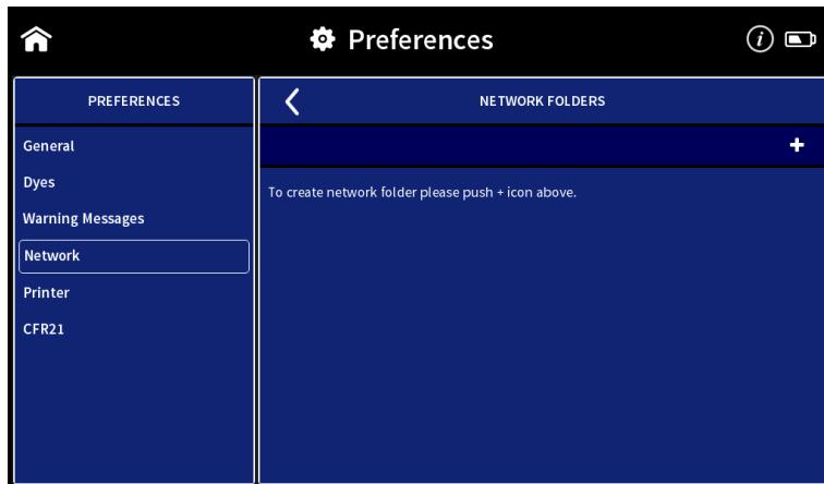
To add a network folder push the + icon and enter network folder nickname and network path of the network folder. If the local network requires authentication enter user name and password for login and if necessary the domain. To save the Network folder push the disk icon (💾).
