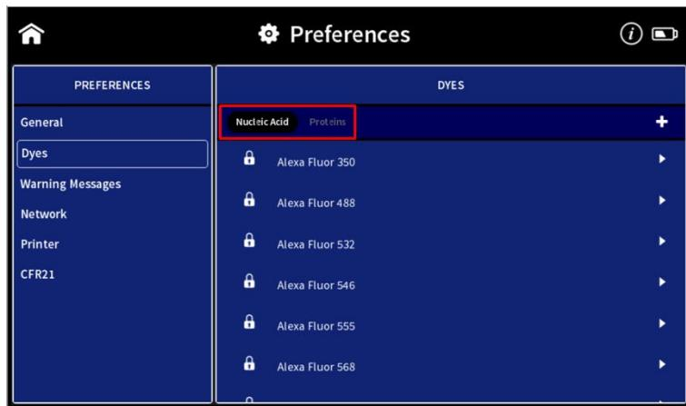
Each dye has either a lock icon (🔒) in front of the dye name indicating that the dye is locked and cannot be changed or a delete symbol (Delete). The delete option is only available for unlocked and not preprogrammed dyes.
