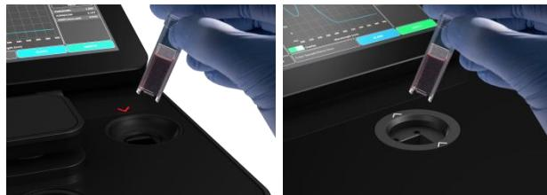
**Note:** For the NP80 the cuvette compartment needs to be activated by the “Change to Cuvette” button in the parameter area. Once the cuvette option is activated the sample compartment door will be opened automatically and a red arrow above the cuvette compartment will appear. The arrow indicates the light path.
