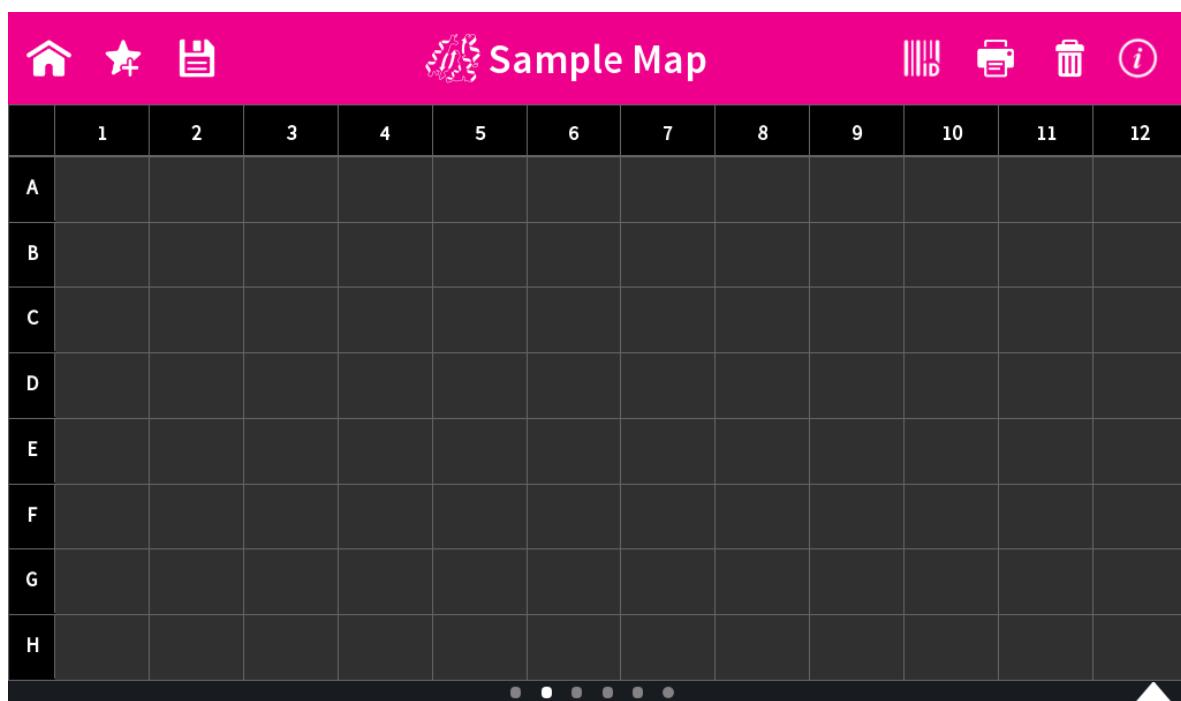
The sample map offers the possibility to select cells and define sample IDs for measurements. It is not necessary to make a selection. If cells are left empty without defined sample IDs for horizontal and vertical sample loading, all 12 positions for horizontal loading and all 8 positions for vertical loading are measured.
