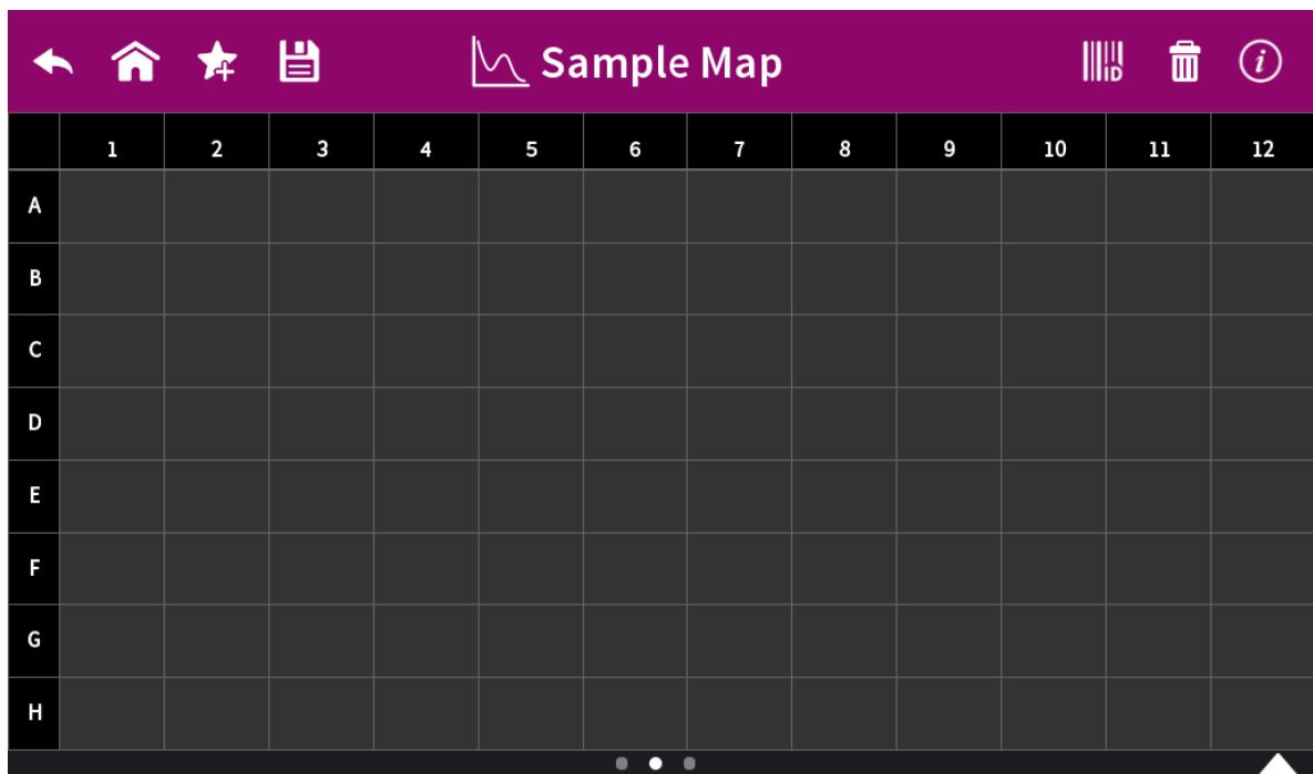
The sample map offers the possibility to select cells and define sample IDs for measurements. It is not necessary to make a selection. If cells are left empty without defined sample IDs for horizontal and vertical sample loading, all 12 positions for horizontal loading and all 8 positions for vertical loading are measured.
