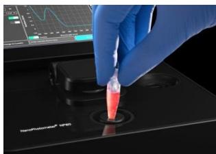
4. Raise the lid arm and pipette the appropriate amount of blank solution onto the illuminated sample window on pedestal. The illumination turns automatically off when the lid arm is lowered.
