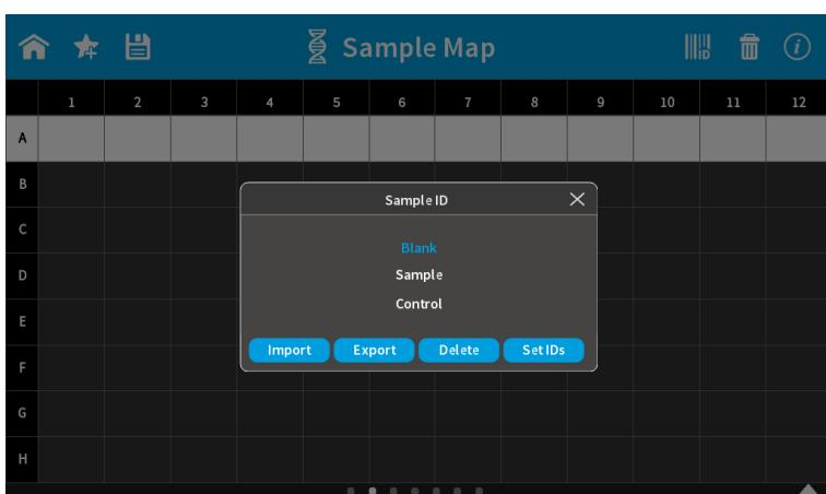
To set sample IDs, select Blank (BLK), Sample (SPL) or Control (CRL) and push on “Set IDs” button. Sample IDs are numbered automatically.
