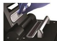
13. Apply samples to the illuminated sample windows on pedestal and press the sample button to initiate the measurement.
