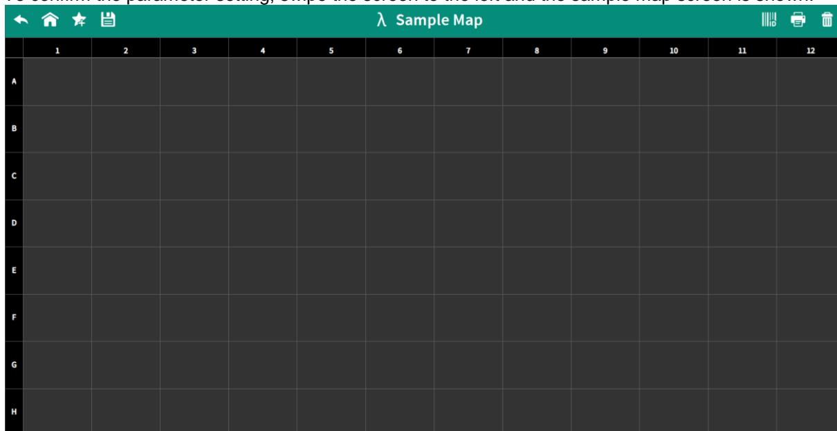
The sample map offers the possibility to select cells and define sample IDs for measurements. It is not necessary to make a selection. If cells are left empty without defined sample IDs for horizontal and vertical sample loading, all 12 positions for horizontal loading and all 8 positions for vertical loading are measured.
