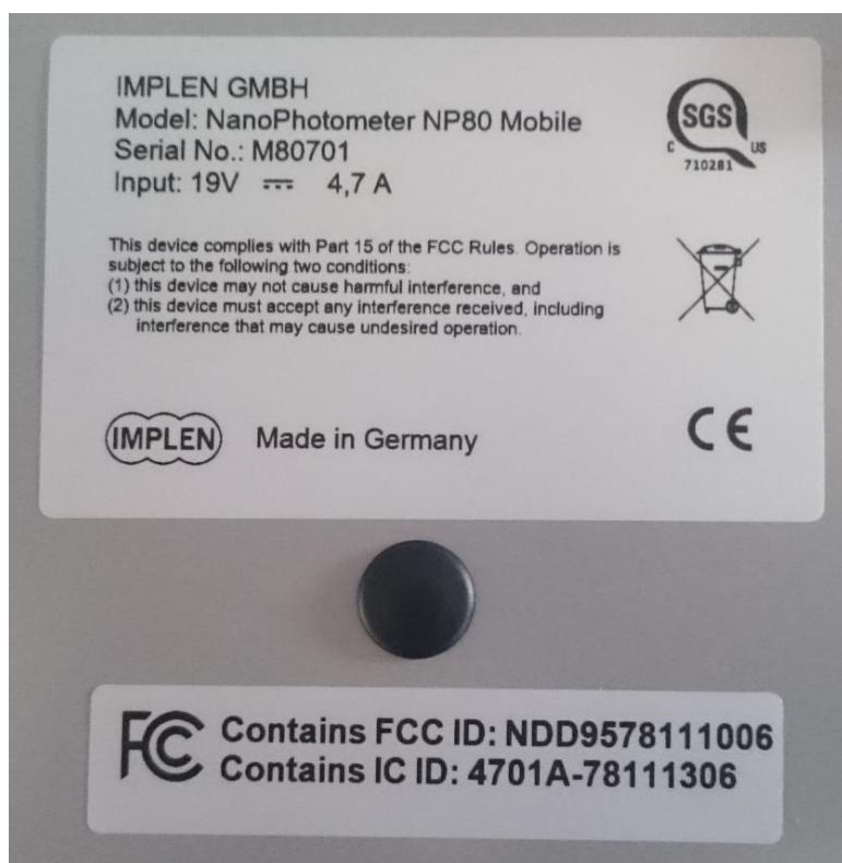
Model name, device serial number and FCC ID are located on the identification plate on the bottom of the instrument.
