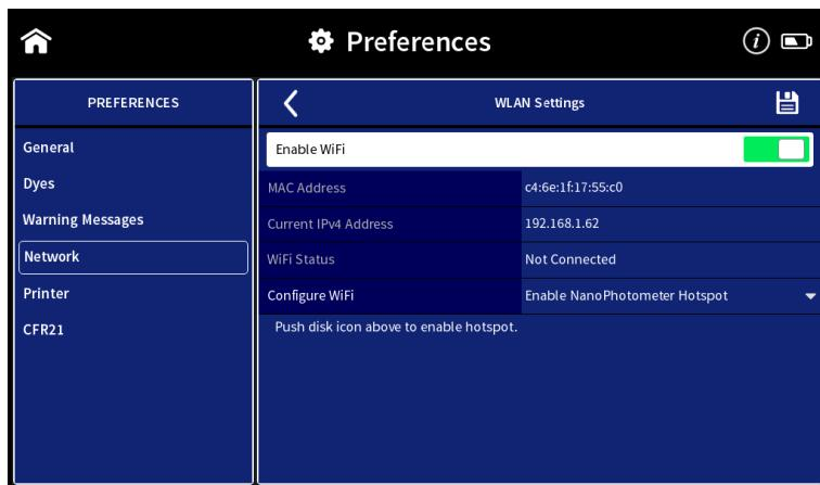
To set up a Wi-Fi® network select “Connect to Wi-Fi® Network” in the dropdown. Select an available Wi-Fi® network from the dropdown list or choose other for hidden networks and enter the password. Confirm with the disk icon (💾).
