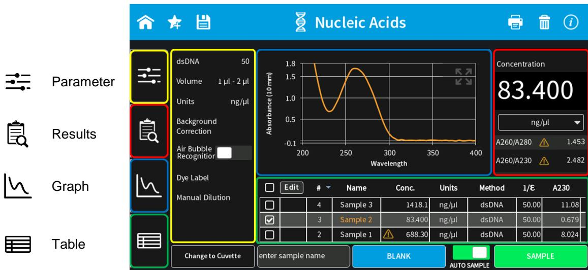
**Note:** There is no tab bar available for smartphone versions. The parameter, results and graph screens are shown full screen. Parameters need to be confirmed (>) to get to the measurement screen. It is possible to toggle between the results and graph area by swiping left and right. There is no table area available for smartphones.
