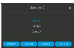
To delete sample IDs, close the pop up, select the row/column for which the sample IDs should be deleted and reopen the sample ID pop up and push the Delete button.
