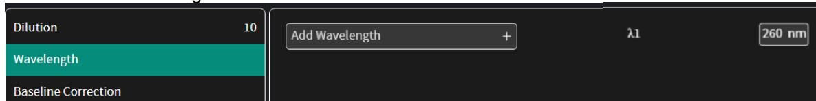
5. Baseline correction is set off by default. Enabling the baseline corrections shows a list with different wavelength options: 377 nm, 604 nm, 650 nm, 770 nm and 823 nm. Option to enter any wavelength between 200 nm and 900 nm.
