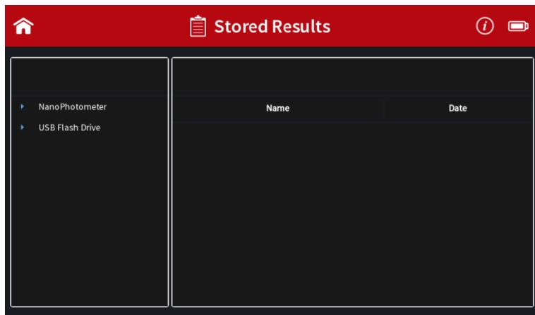
On the left side of the screen all available directories/storages are shown: NanoPhotometer®, Control Device, Network and/or USB flash drive (depending on availability). By tapping on a storage folder, the subfolders of this storage folder will be shown on the left side and the individual files on the right side. On the right side of the screen all saved result files of the selected folder are shown and can be opened by a long or double click.
