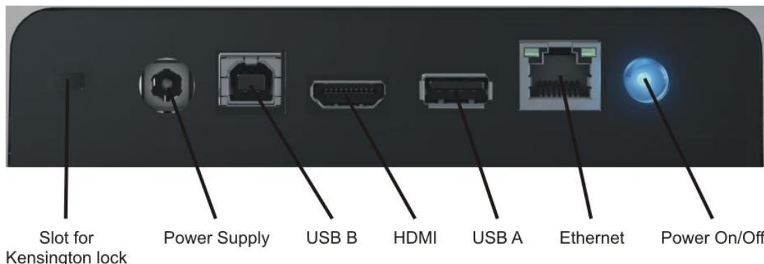
To boot/shut down the NanoPhotometer® push shortly (< 1 second) on the power on/off button at the back of the NanoPhotometer®.
