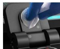
13. Apply sample to the sample window on pedestal and press the sample button to initiate the measurement.
