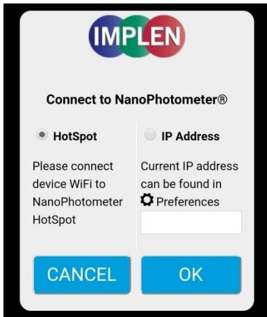
4. When connected the NanoPhotometer® will recognize the tablet/smartphone as a remote control device and measurements can be initiated from the tablet or smartphone.
