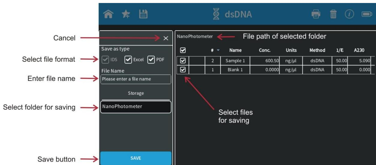
By default all samples are ticked in the first column of the table and will be saved. It is possible to select samples for saving by using the tick boxes. The header tick box selects/deselects all samples.
