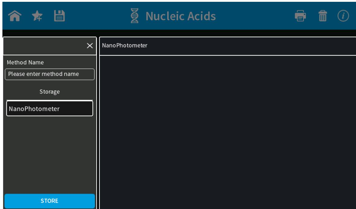
Enter a method name and select a save location in the folder. Options include: NanoPhotometer®, USB flash drive (if connected) and Network folder (if defined). Push the store button to save the method.
