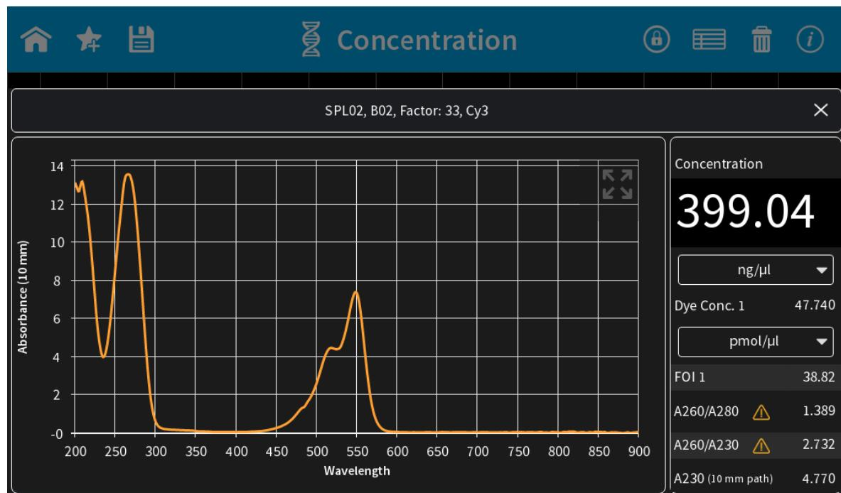
A double click to a result cell shows tick boxes for all measured samples. The tick boxes can be used in the graph screen to overlay up to 12 samples. Up to 12 ticked samples will be overlaid by pressing the graph icon ( in the navigation bar.
