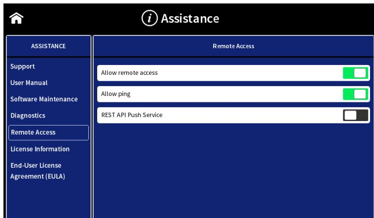
Remote access and ping are active after booting the NanoPhotometer® and are automatically switched off after 15 minutes. A renewed activation for remote access is possible for 30 minutes at a time. The activation of ping remains active until the next restart of the NanoPhotometer.
