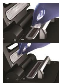
11. Apply samples to the illuminated sample windows on pedestal and press the sample button to initiate the measurement.
