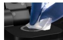
**Note:** It can be helpful to apply the blank a second time and read it as a sample to ensure a proper blank.
