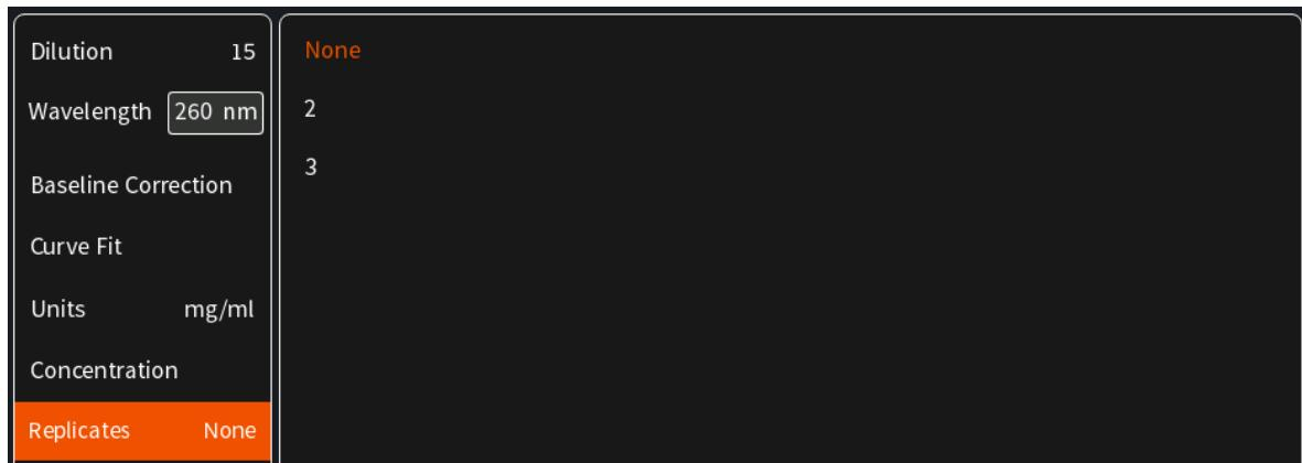
9. Once Standard curve is created or loaded it will be used for concentration calculations in the method. It might be necessary to do a blank measurement.
