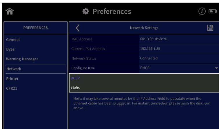
For static IP configuration select Static in the Configure IPv4 dropdown and enter the IPv4 address, netmask and gateway then confirm with disk icon (💾).
