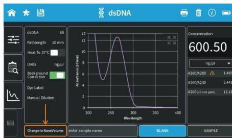
**Note:** If there is no “Change to NanoVolume” button available in the method go to preferences/general and enable the NanoVolume option. We guarantee our submicroliter cell specifications only for Implen submicroliter cells which are aligned to the NanoPhotometer® C40 by Implen.
