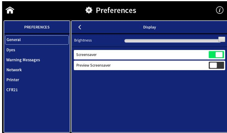
Screensaver: Option to switch the screensaver video on and off. With Preview Screensaver the screensaver can be started immediately.
