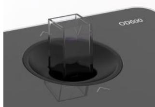
Initiate a blank measurement with the blank button.
