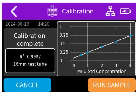
**Note:** The default 16mm tube calibration curve was generated using the McFarland standards set from Company ProLab, Serial Number 395123, traceable to 260-140 SD2350.
