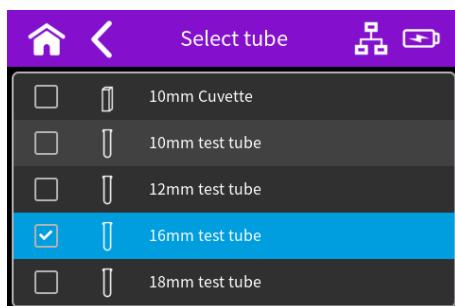
The default tube type for McFarland measurements is the 16 mm test tube. Implen has factory-set a 16mm test tube calibration curve, which can be overwritten, which will be reset after a factory calibration.
