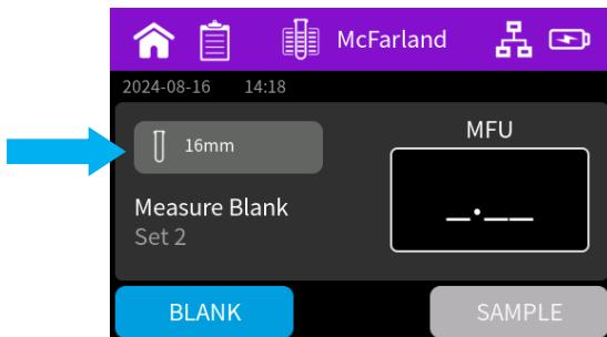
**Note:** The default 16mm tube calibration curve was generated using the McFarland standard set from Company ProLab, Serial Number 395123, traceable to 260-140 SD2350.
