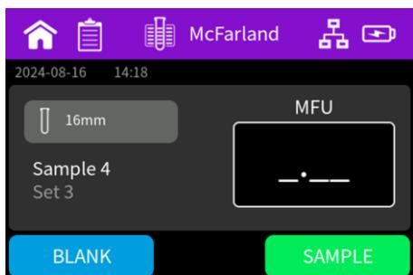
Initiate a sample measurement with the sample button. Upon completion of measurement remove the cuvette.
