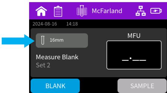
Note: The tube type selection in the McFarland app is intended solely for labeling purposes and does not dictate the specific tube size required for calibration with the standard curve. It is not mandatory to use the indicated tube type; however, for accurate and reliable results, it is essential to use the same tube type consistently across calibration, blank, and sample measurements.
