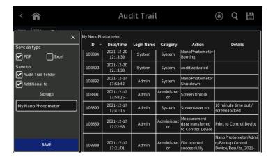
The audit trail folder can only be accessed by Administrators and Viewers via file server access. The folder NanoPhotometer\_Admin contains all relevant files including the audit trail. Connection options are LAN/WLAN, USB cable or Wi-Fi® (WiFi) Hotspot.
